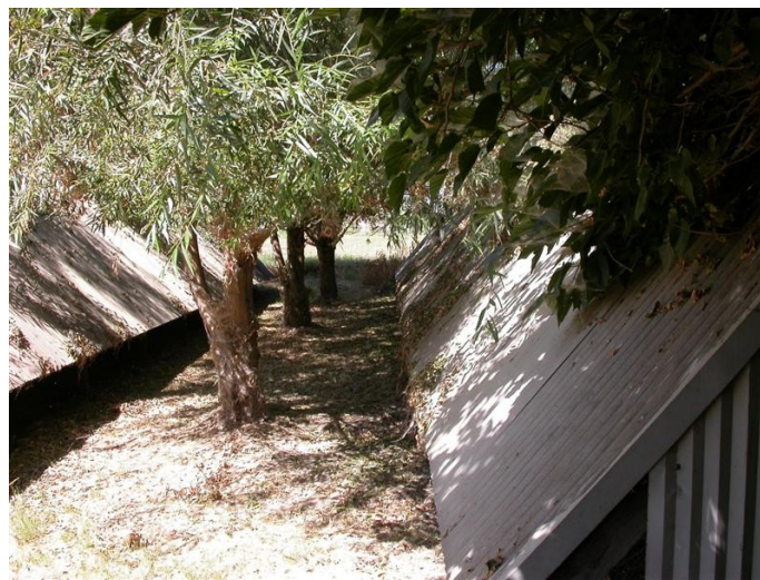
Figure 6. Trees planted between the A-frame barns provide shade to cool the barns and ground around them.
